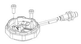
Insert O-Ring (60x2mm) Pos.1 into the sealing groove.
