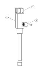
Mount the speed sensor with the gearbox-specific mounting kit onto the input shaft of the gearbox and fix the cable routing according to the specifications of the mounting kit. The speed sensor must be set to a sensing distance of 5 mm.
