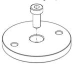
5. Attach sensor interface to mounting adapter (M6x14).
