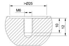
Clean the attachment surface and protect it from corrosion with suitable aids.  Attach the mounting adapter with cylinder head bolt (M6x14), paying attention to the orientation.
