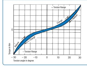
Due to the specific construction characteristics of the ROSTA rubber suspension element, pivoting the device  $\pm$  results in a slightly progressive spring characteristic. The torsion angle is limited to  $\pm$  30 for most elements.
