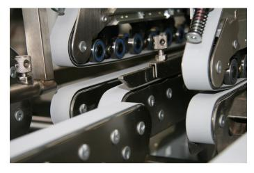
RAPPLON® Folder Gluer Belt 'QuickSplice' design: long term measurement on premium brand high speed folder gluers under working conditions confirm reduced energy consumption of up to 14% - immediately after installation and throughout the lifetime of the belts.
