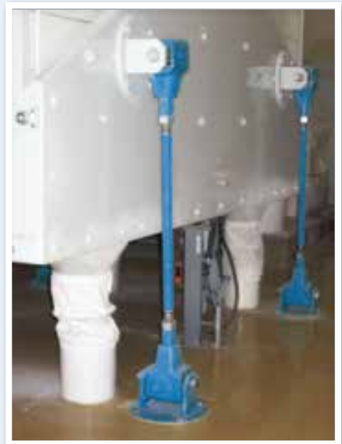
Free oscillating gyratory sifter for the flour selection on 8 pcs. AV 38 elements
