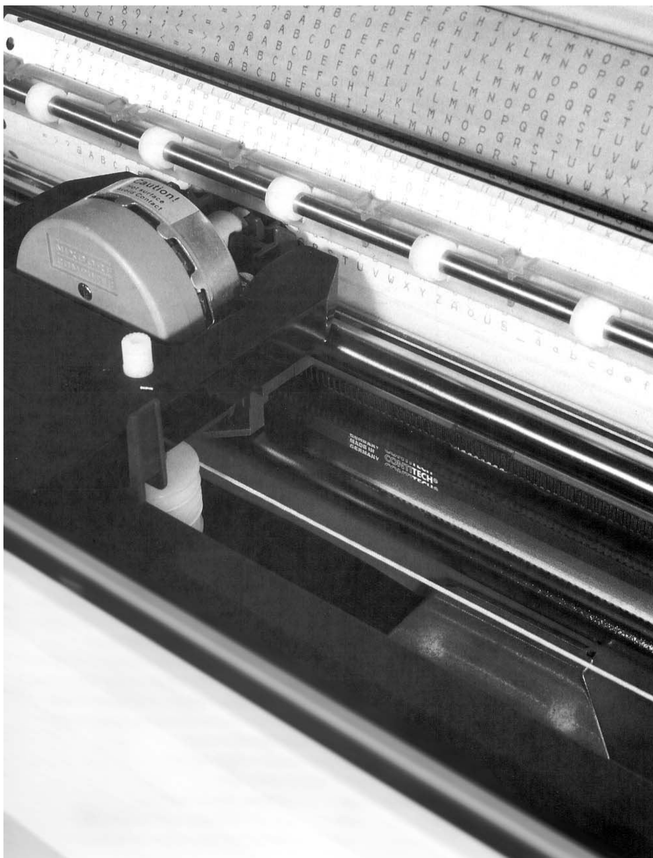
CONTI SYNCHROBELT® synchronous drive belt on a printer
